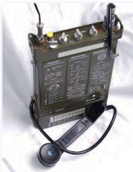
Fig. 5: The RF10 transceiver with microphone, whip antenna and battery pack attached.
