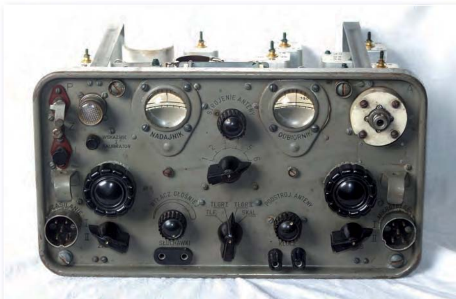
Fig. 2: The RBM-1 transmitter receiver, transmitter tuning on the left and the receiver tuning on the right.
