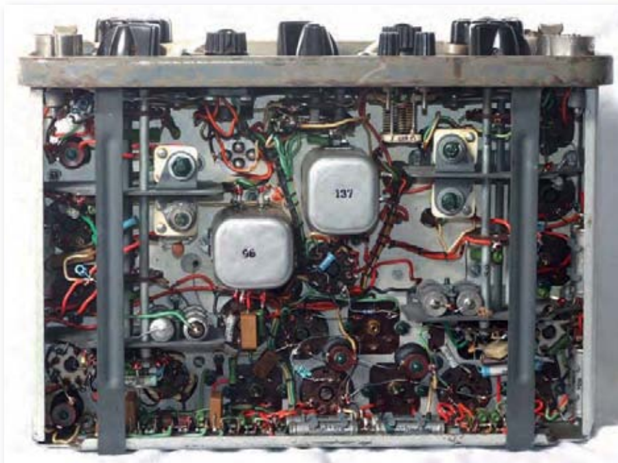
Fig. 4: Underside of RBM-1, transmitter stages on the left, receiver stages on the right and bottom section.
